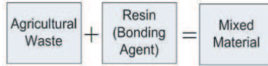
Figure 2. The process flow for the mixing of the materials for the fabrication of the rice husk particle board.
