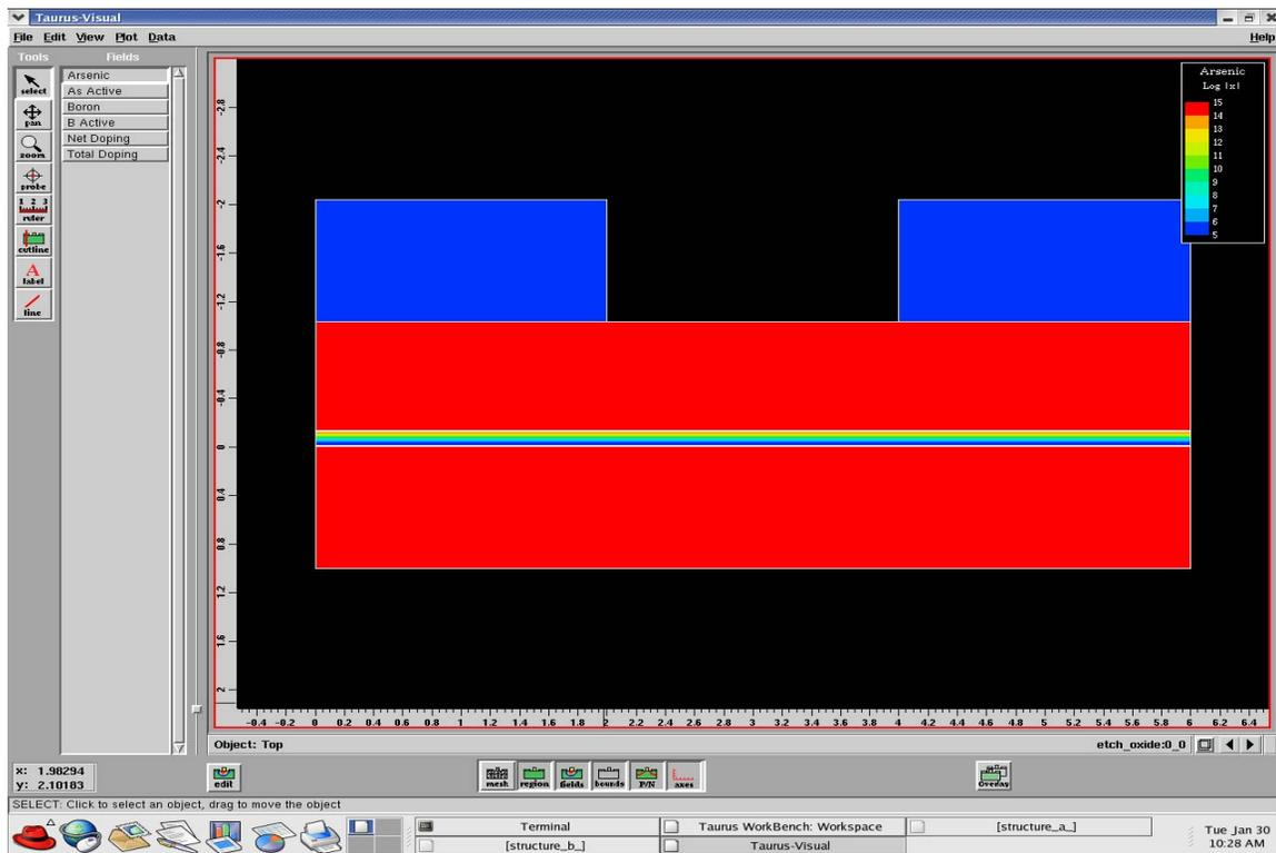
10 The last stage is diffusion process or annealing process (structure B)
