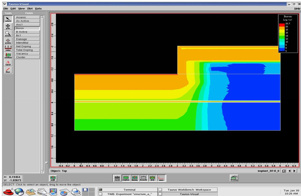
8. The last stage is diffusion process or annealing process
