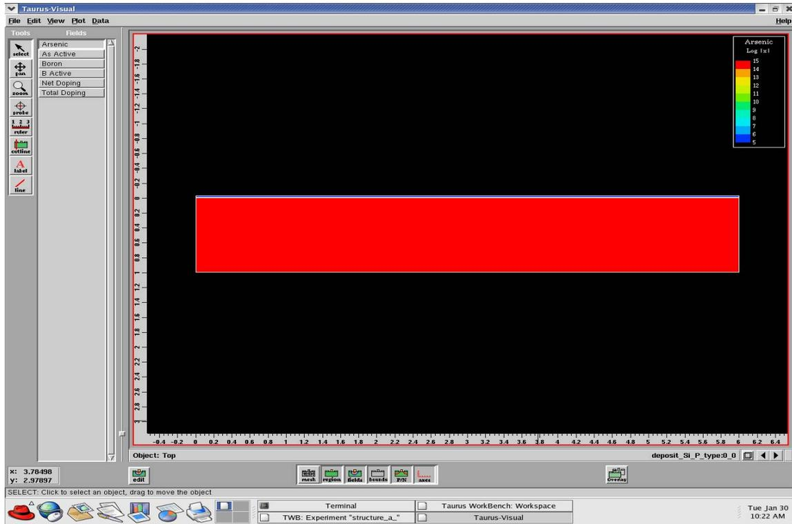
3. Silicon doped Arsenic is deposited on top of the silicon doped Boron underling layer
