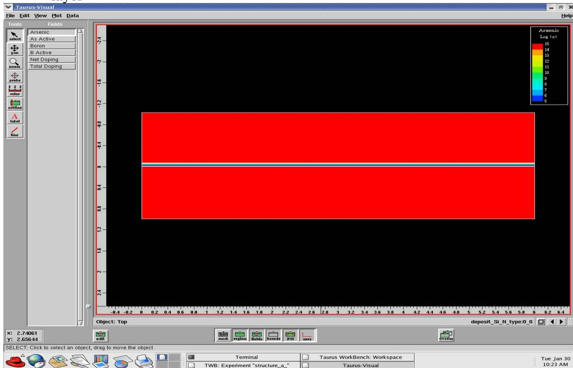
4. A silicon oxide layer is grow on top of the silicon doped Arsenic layer
