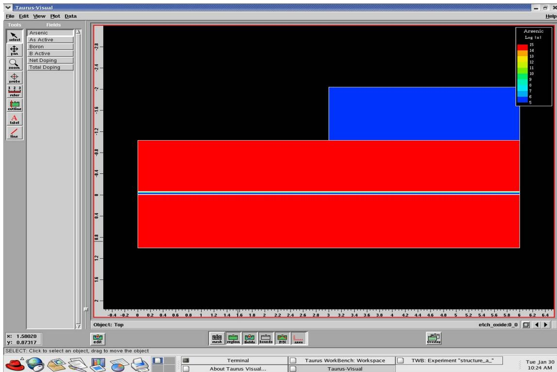
6. After that the Boron will implant into the structure
