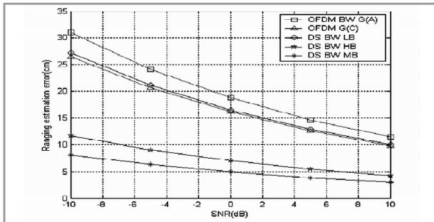
Figure 1: Ranging error based on the CRLB for various types of UWB IEEE802.15 standards
