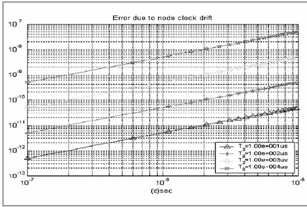
Figure 7: Ranging Error with a single TWR between the node and cluster-head estimation
