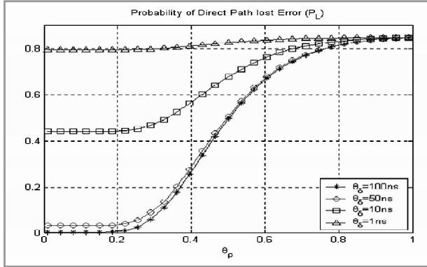
Figure 2: Probability of a direct path lost error ( $P_L$ ) with a peak SNR of 18 dB
