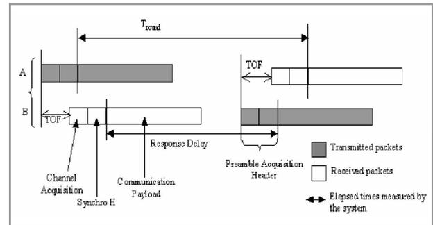
Figure 6: Two-way Ranging (TWR) transaction enabling to estimate the round-trip Time-Of-Flight between two asynchronous terminals (feeding TOA-based positioning algorithms)
