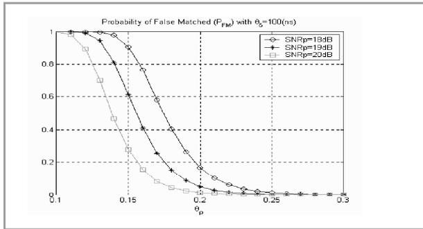
Figure 3: Probability of false matched ( $P_{FM}$ ) with delay threshold ( $\theta_\delta$ ) 100nsec
