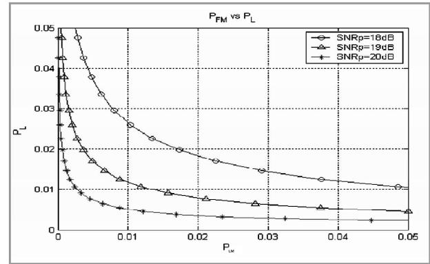
Figure 5: False matched probability versus probability of direct path lost for different peak SNRs.
