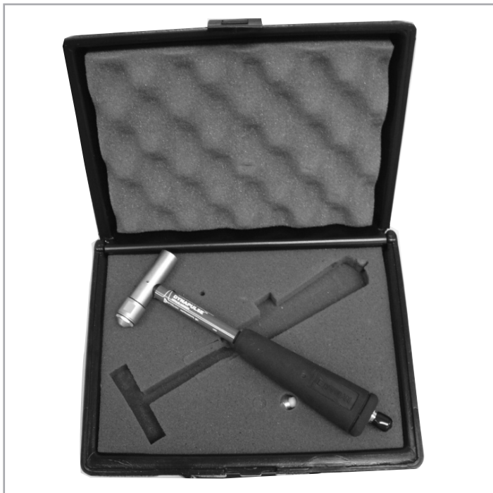
Figure 6: Instrumented hammer for the experimental modal analysis
