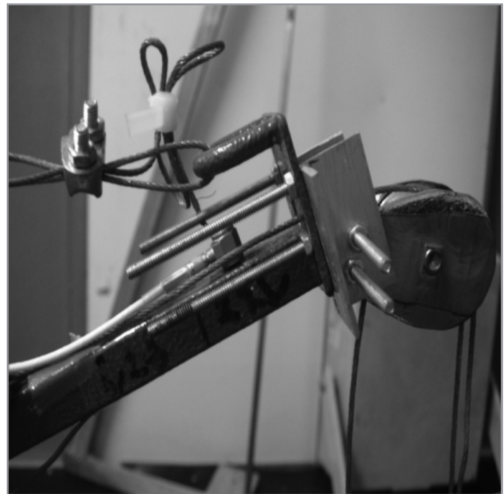
Figure 7: Accelerometer attached to the boom tip to measure dynamic response
