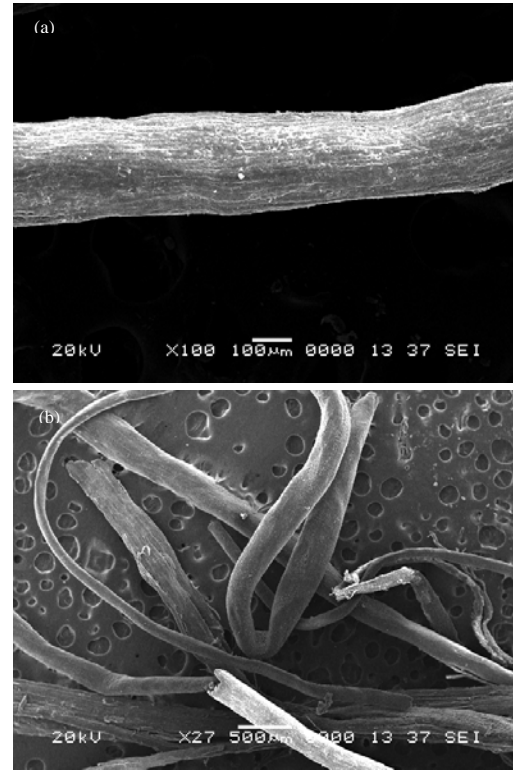
Fig. 2: a) SEM image of coconut fibre at ×100; b) SEM image of coconut fibre at ×500
