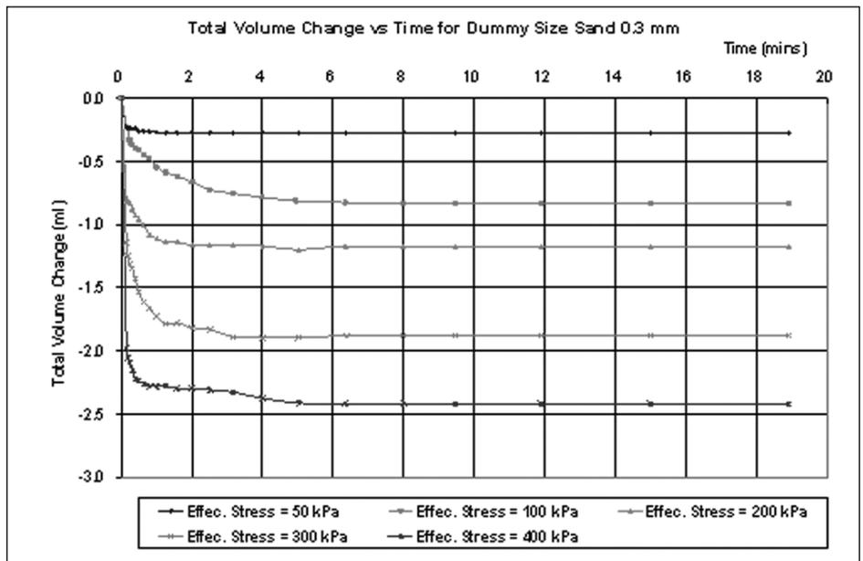
Figure 4: Total volume change during isotropic compression for grain sizes (0.3 mm)
