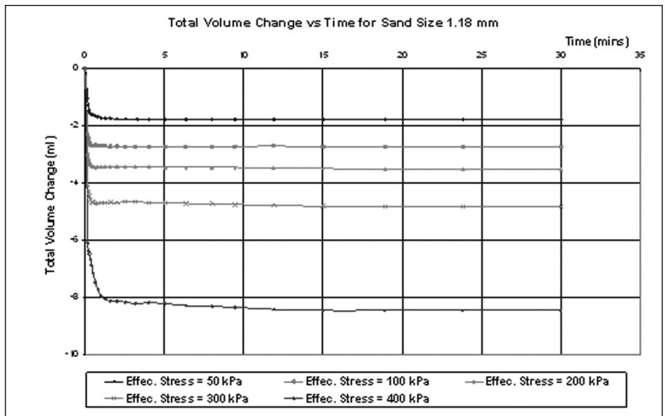
Figure 6: Total volume change during isotropic compression for grain size (1.18 mm)
