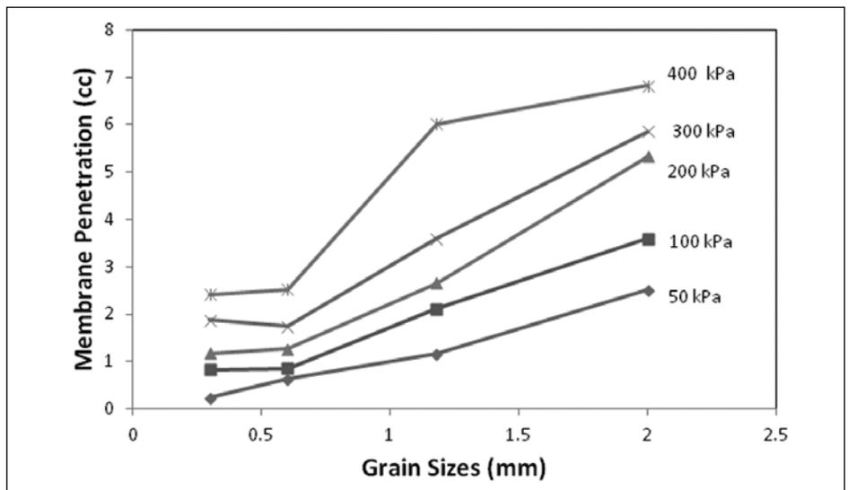
Figure 12: Comparison of membrane penetration relation to grain sizes (0.3, 0.6, 1.18 and 2.0 mm) under different effective confining stress (50 – 400 kPa)
