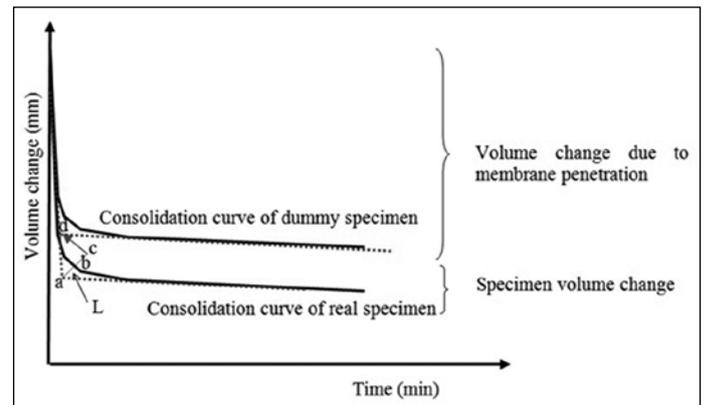
Figure 1: Schematic diagram to estimate membrane penetration isotropic consolidation curve
