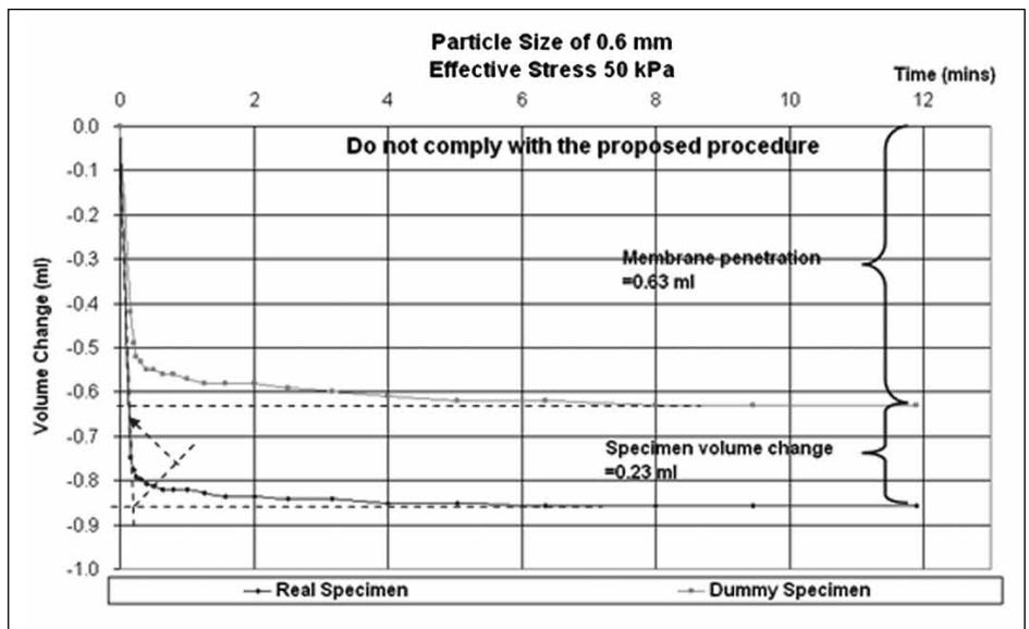
Figure 9: Graphs of isotropic consolidation on the dummy and real specimens of grain size 0.6 mm and effective stresses of 50 kPa
