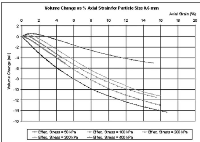
Figure 14: Volume change for specimen of particle size 0.6 mm
