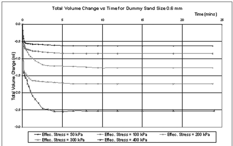
Figure 5: Total volume change during isotropic compression for grain size (0.6 mm)
