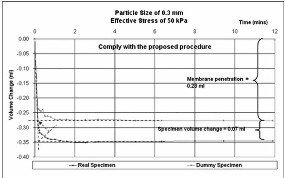
Figure 8: Graphs of isotropic consolidation on the dummy and real specimens of grain size 0.3 mm and effective stresses of 50 kPa
