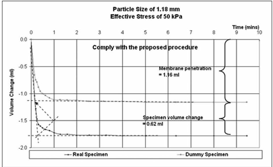
Figure 10: Graphs of isotropic consolidation on the dummy and real specimens of grain size 1.18 mm and effective stresses of 50 kPa
