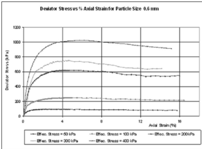
Figure 13: Stress-strain curve of specimen of grain size 0.6 mm
