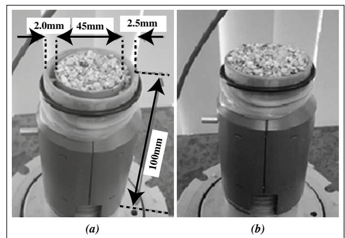
Figure 3: Dummy specimen with rigid cylindrical core (a) Sand particles were placed over and around the rigid core (b) Fully prepared dummy specimen for particle size of 2.0 mm
