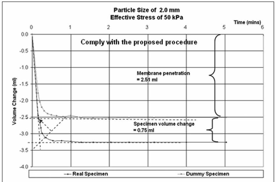
Figure 11: Graphs of isotropic consolidation on the dummy and real specimens of grain size 2.0 mm and effective stresses of 50 kPa
