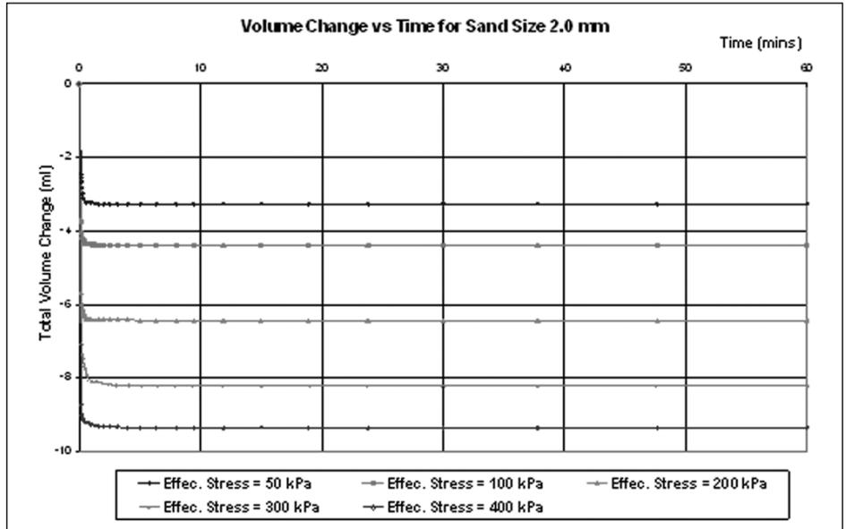
Figure 7: Total volume change during isotropic compression for grain sizes (2.0 mm)
