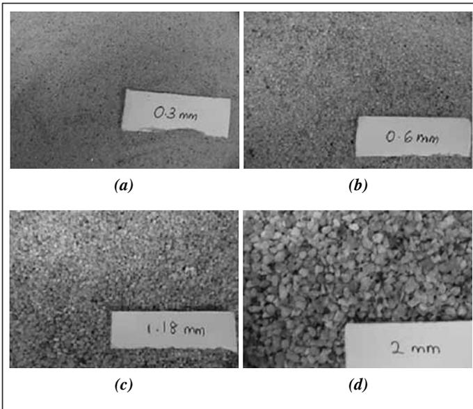
Figure 2: The four sizes of quartz sand as the test materials of diameter (a) 0.3 mm (b) 0.6 mm (c) 1.18 mm and (d) 2.0 mm
