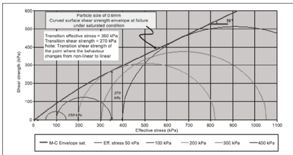
Figure 15: Curved surface shear strength envelope at saturation for particle size of 0.6 mm
