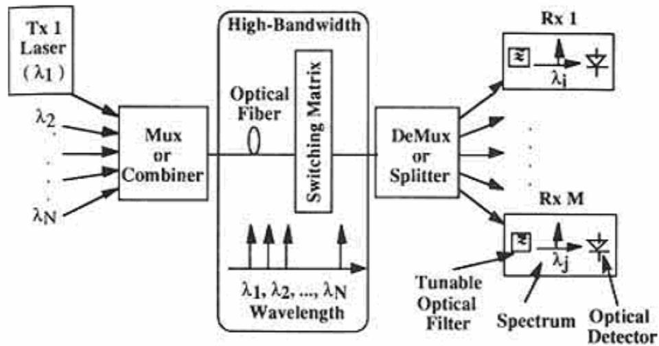
Figure 2.4: Diagram of a Simple WDM System
