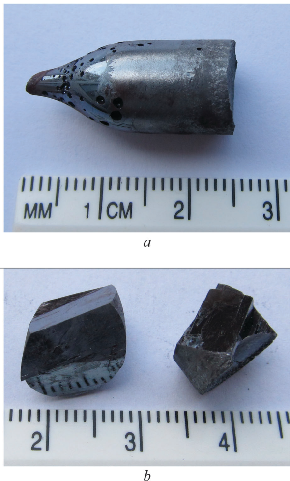
Fig. 3 Panoramic view of the as-grown (a) \text{Tl}_{0.8}\text{In}_{0.8}\text{Sn}_{0.2}\text{Se}_2 and (b) \text{Tl}_{0.9}\text{In}_{0.9}\text{Sn}_{0.1}\text{Se}_2 single crystals.
