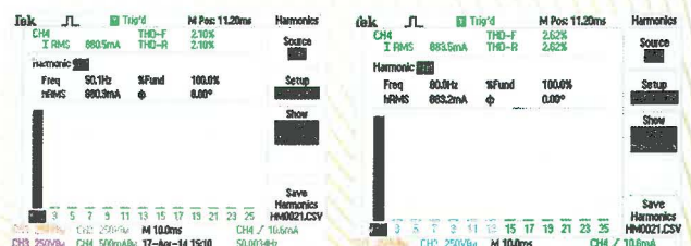
Figure 5: Current harmonic profile for 50Hz and 80Hz with multiple switching angles
