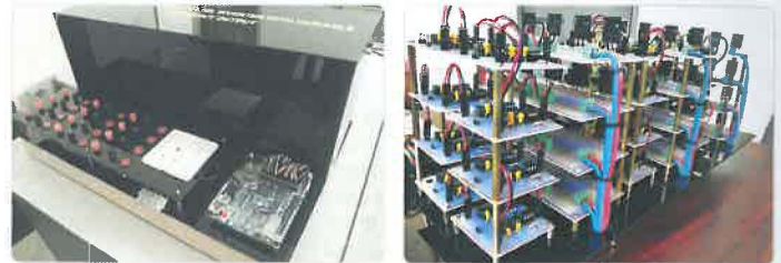
Figure 1: Three phase multilevel inverter
