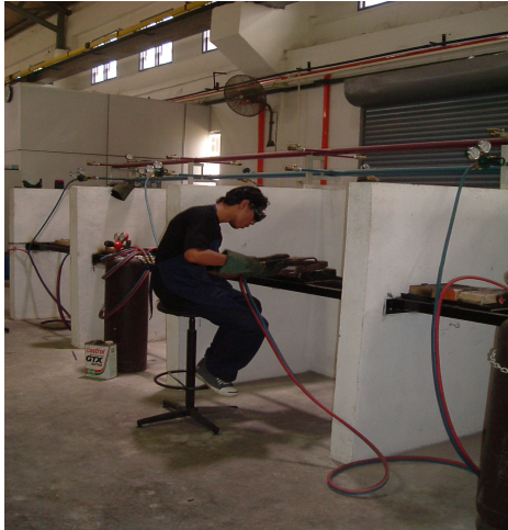
Fig.7 Gas welding work
