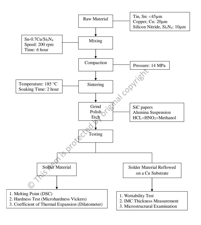
Figure 1.1: The complete flow chart of the project.
