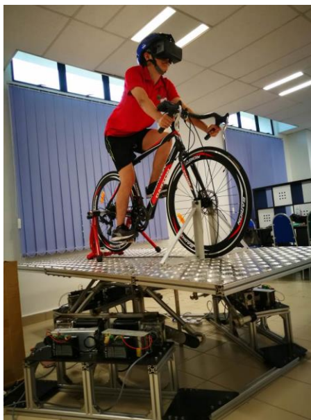
Figure 8: User testing the spatial immersive track cycling simulator
