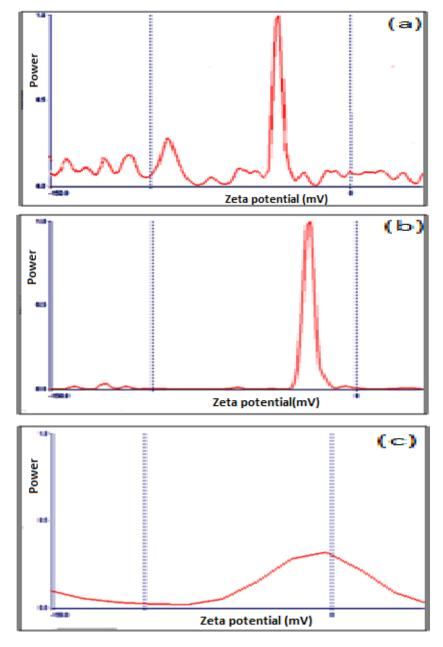
**Figure 4.** ζ-potential of silver NPs prepared by laser ablation in acetone, toluene, and cyclohexane, respectively.
