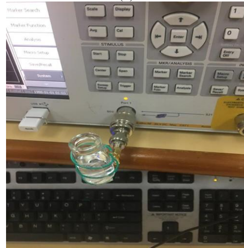
Fig. 2. Simple Helical Antenna. (a) Helical antenna (b) helical antenna design using CST (c) Helical antenna under test with an empty bottle.
