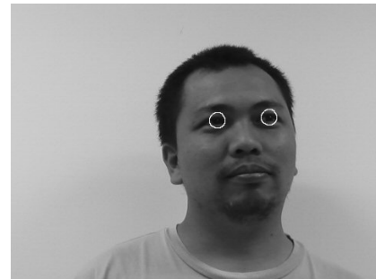
Figure 1. The positions of the irises of both eyes detected by the iris detection algorithm from input image
