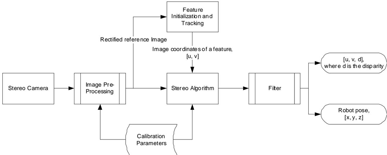
Fig. 2. The vision system for a SLAM implementation [32]
