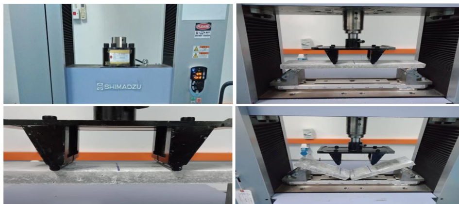
Figure 2. Third point loading procedure.
