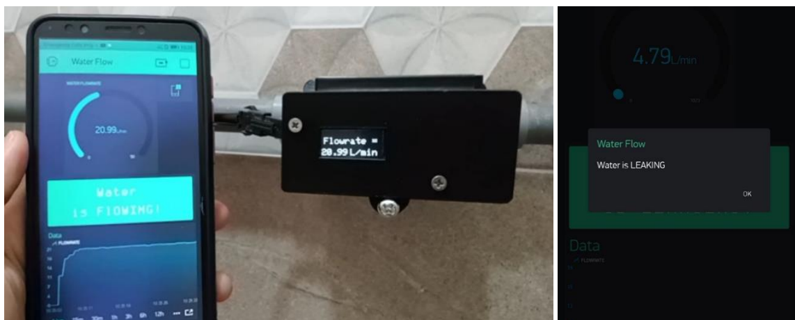
Figure 8. Results from the receiver and leakage notification from the Blynk apps
