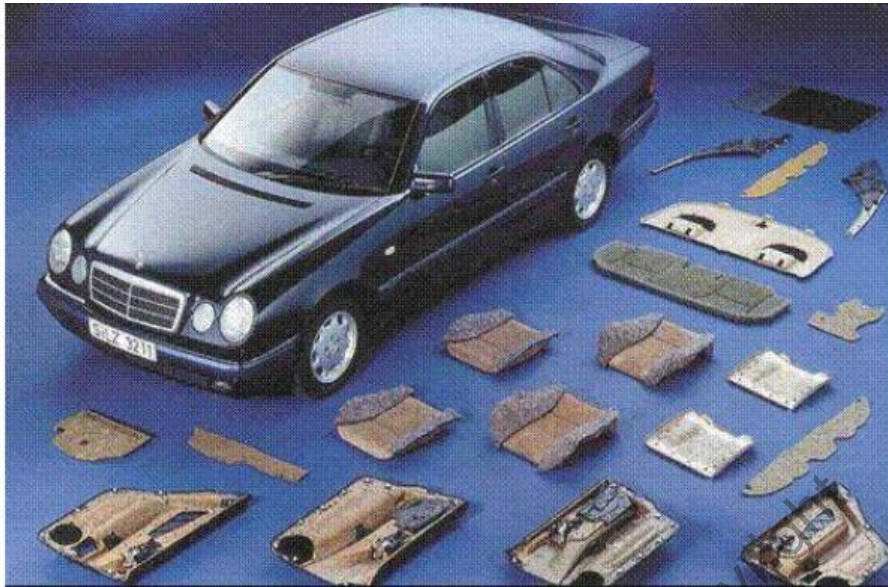
Figure 1.1 : Mercedes-Benz with flax thermoset door panels
