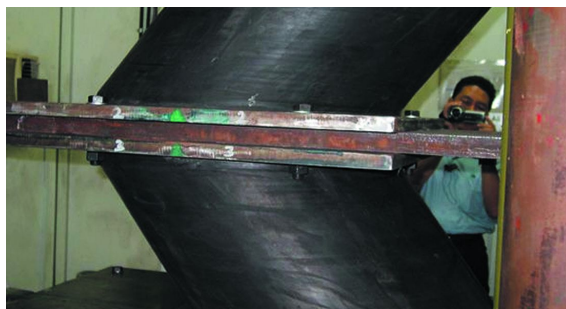
Figure 3: A pair of the Iranian bearings being simultaneously compressed and sheared at a cyclic rate of 0.004Hz
