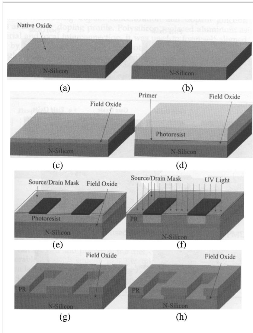
**Figure 3.1** Fabrication Process step (a) and (b) process wafer cleaning using BOE (Buffered Oxide Etch). (c) An oxidized Si wafer by wet oxidation. (d) Application of resist. (e) and (f) Resist exposure through the mask. (g) The wafer after the development. (h) The wafer after  $\text{SiO}_2$  removal.
