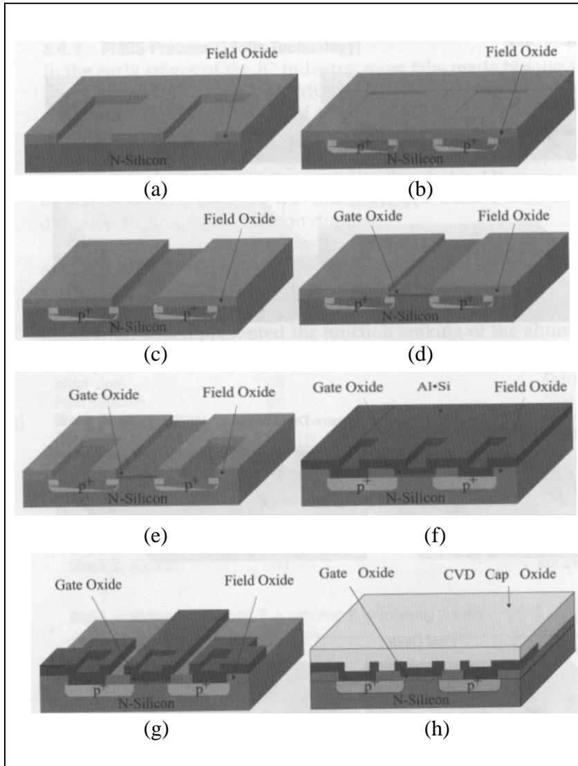
**Continue: Figure 3.2** Fabrication process step (a) after strip photoresist using acetone. (b) source/drain doping. (c) Form gate pattern using lithography process. (d) Grown gate oxide using dry oxidation. (e) Form contact pattern (f) deposit metal (aluminum) using PVD. (g) After aluminum etch. (h) Deposited passivation layer.
