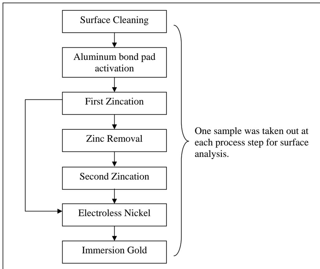
**Figure 3.3.** Process sequence for electroless nickel immersion gold deposition.
