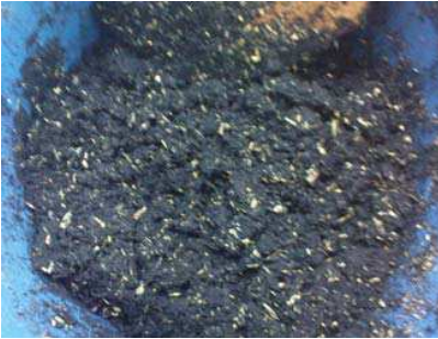
Figure 3. Mixture of 75 percent rubber tire dust and 25 percent rice husks.
