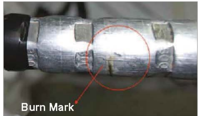
Figure 2: Burn mark at the ferrule (R-phase)
