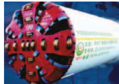
Pipe jacking (Tunnelling machine for rock)
