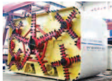
Rectangular Pipe jacking machine
