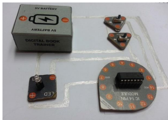
Figure 5. Circuit connection on the digital electronic book trainer.
