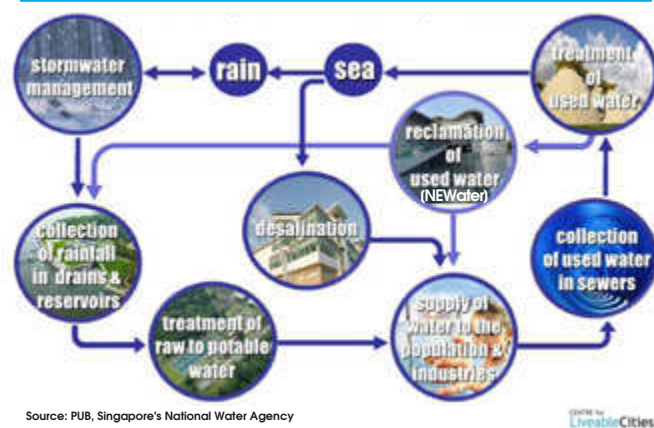
Figure 4: Closing the water loop (Source: PUB)
