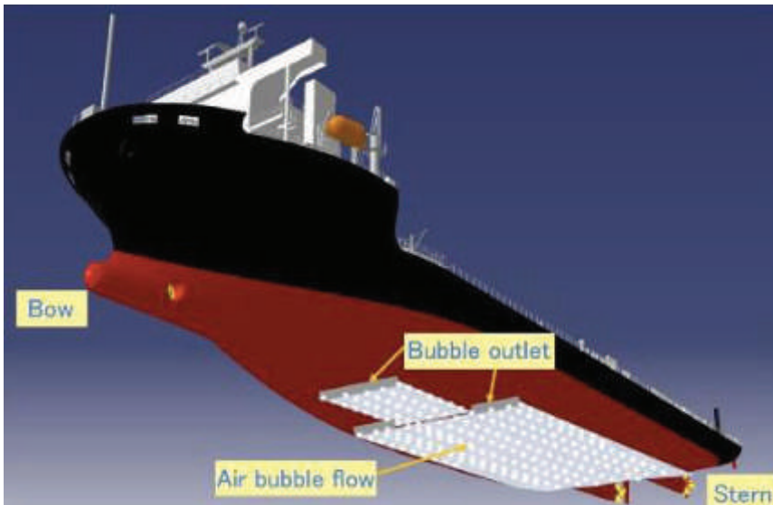
Figure 9: Ship Air Lubrication System
