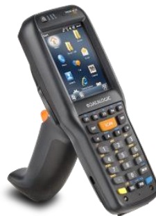
Figure 4. Handheld barcode reader and mobile computer terminal [13].
