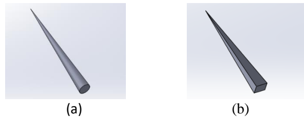
Figure 2. The 3D design of the microneedle; (a) conical design (b) pyramid design.
