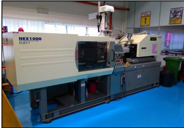
Fig. 3. Injection Moulding Machine, Nissei NEX1000.
