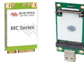
Fig. 5. Wireless internet with mini PCI-E to USB adapter.
