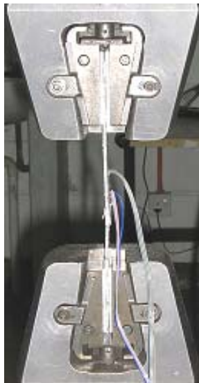
(b) Installed with strain gauges
