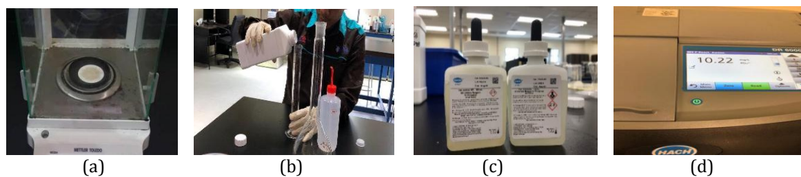
Figure 3. Preparation of the synthetic aqueous solution, (a) Weighed the \text{KH}_2\text{PO}_4 , (b) Dilution process (c) Phosphate, Reactive (Orthophosphate) Amino Acid Method, and (d) DR6000 UV Spectrometer.
