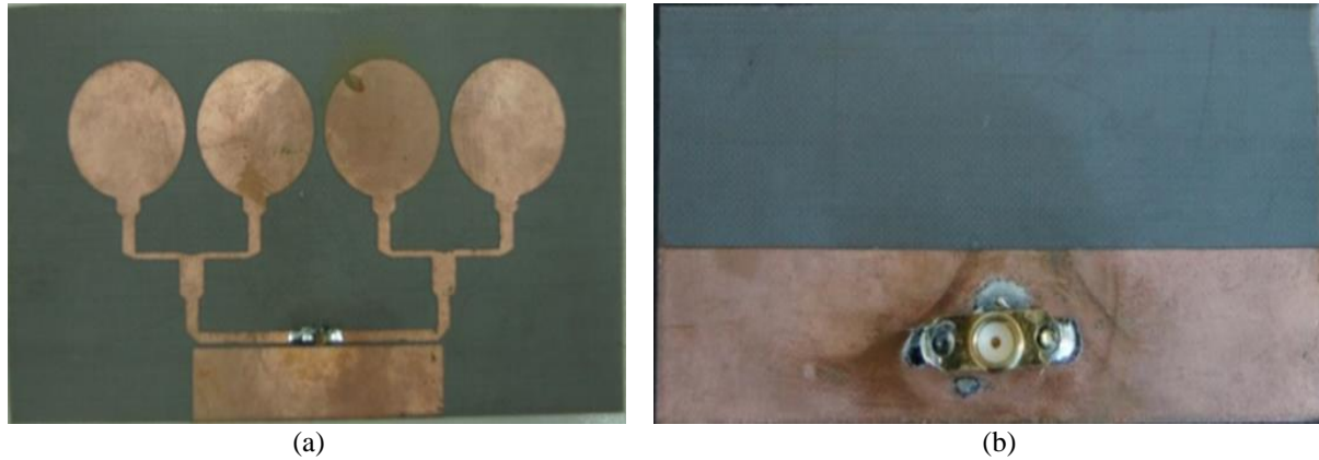
Figure 2. Fabricated UWB array antenna. a) Front view, b) Back view.
